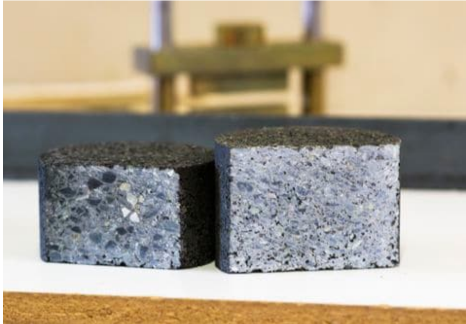
These samples show a product using recycled asphalt and G5 polymer from TechniSoil Industrial, a plastic-roadway company. (TechniSoil Industrial)
